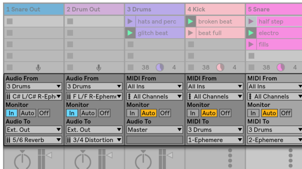
Tracks Feeding MIDI to and Tapping Audio From the Parts of a Multi-Timbral Instrument.
